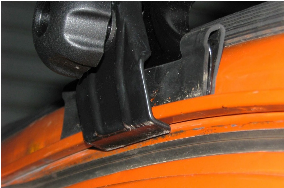
Photo 4 above shows the adjustable clamp of the mount firmly wrapped underneath the gutter. This locks the gutter solidly between the upper mount and the lower clamp, holding the steel mount "welded" in place on the vehicle.
