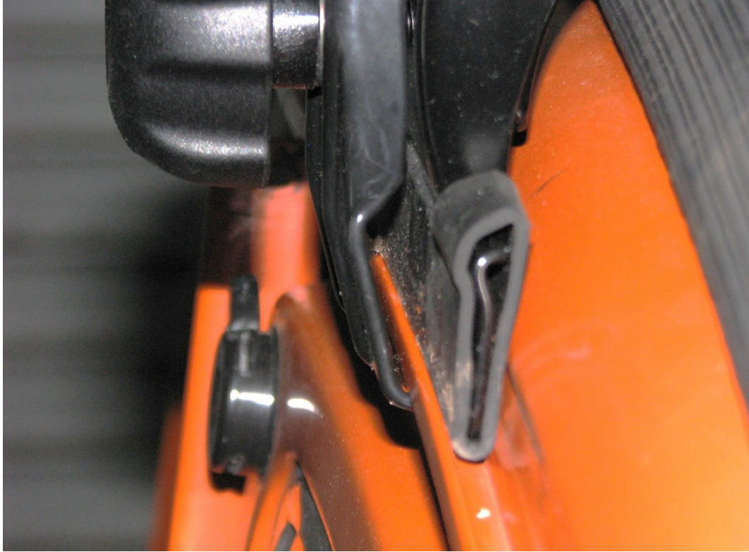
Photo 3 above shows one end of a rubber-sleeved steel mount sitting in the rain gutter, hard against the bottom of the gutter where it normally travels. The mount can't move sideways once locked in place and the rubber sleeve ensures the steel mount does not damage the vehicle paintwork.
